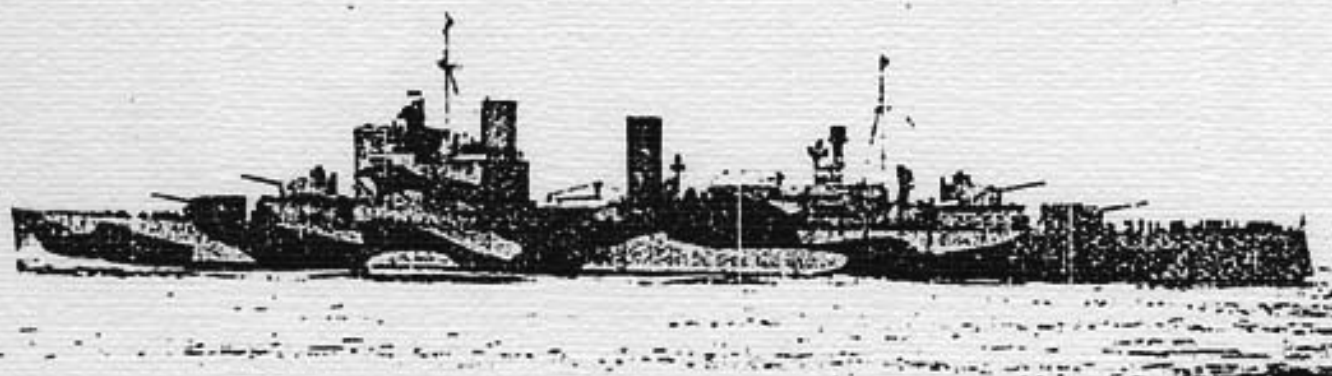
H. M. S. London is the only British heavy cruiser given a modernization to date. A new style block-bridge and re-trunking of the boiler uptakes into two upright stacks replaced the old open bridge and three raking thin stacks. She can be distinguished from the Fiji class by a flush deck hull and twin turrets.
